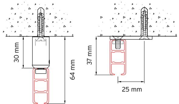
Ceiling mounting with mini suspension hanger
